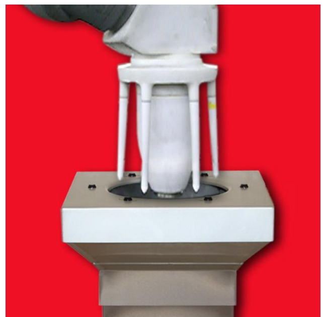
The Applicator Cleaner cleaning an externally charged applicator.
